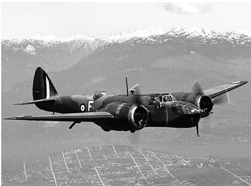
(Image above) The Bristol Fairchild Bolingbroke was a maritime patrol aircraft and trainer used by the RCAF during WW2. It was a license-built version of the Bristol Blenheim MK IV bomber.
